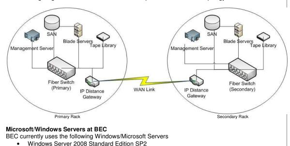
The following diagram shows an illustration of the replication and failover topology
